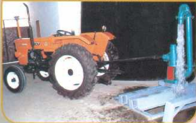
Tractor mounted with deep well turbine can draw water from depths of 800 feet.
